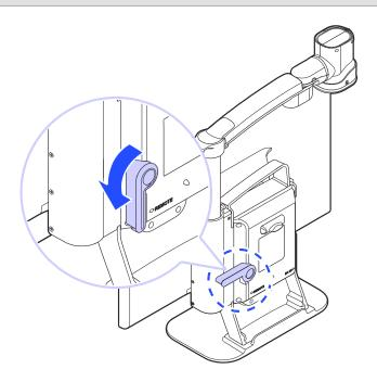
4. Adjust the location of the camera by rotating the camera arm.
